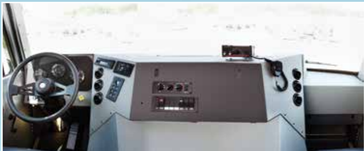
A formed aluminum dash assembly with a rugged finish is standard on the 3000 Model and is an option on the 4000 Model.
