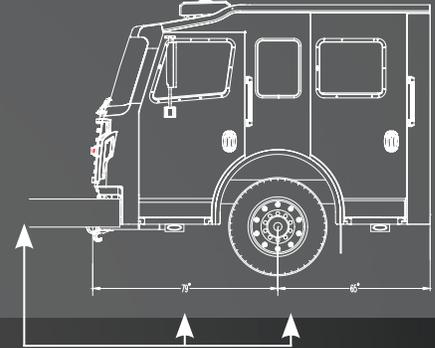
79" Dimension is from "Face of Grille to Centerline of Front Axle."
